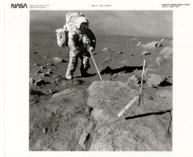
Figure 4.1.2: Harrison H. Schmitt working with a lunar scoop next to a Gnomon on a rock. (NASA photographs)
