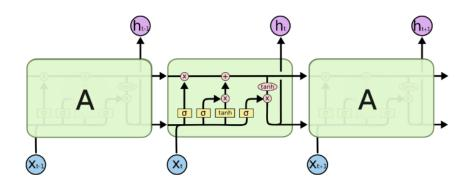
Fig. 3.2 The repeating module in an LSTM contains four interacting gates
