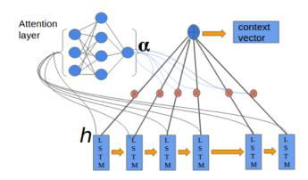
Fig. 3.4 The attention mechanism added on top of LSTM layer.
